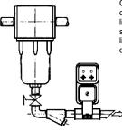
Connect the drain discharge line to the outlet connection on the valve. Run the drain discharge line to a suitable drain or Oil/Water Separator system. If flexible tubing is used, secure the drain line to prevent it from "whipping" when the drain discharges.
